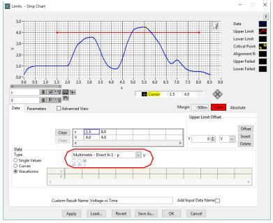
Figure 29-24: Limits On Strip Chart Waveform
