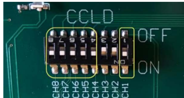
Figure 4-6: Internal CCLD DIP Switches
